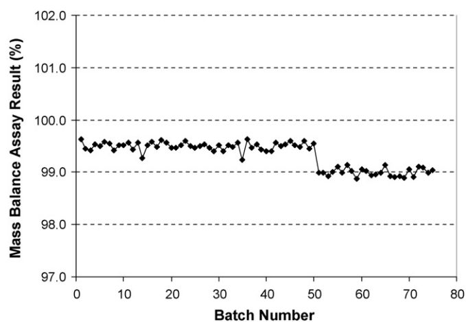
Fig. 5. Simulation of a 0.5% decrease in purity process mean at batch 50 with mass balance assay standard deviation of 0.08%.
